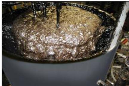
**SECONDARY FLOTATION CELLS**
