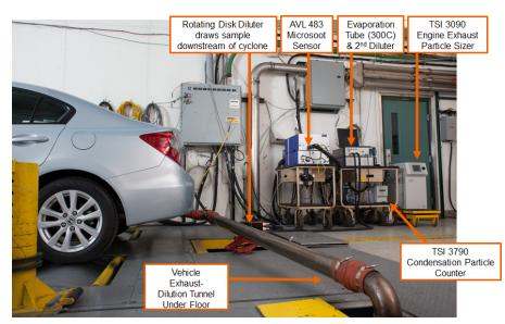
SGS Environmental Testing Corporation has made a significant investment in particulate matter (PM) instruments and measurement techniques for the development of next-generation engines.
