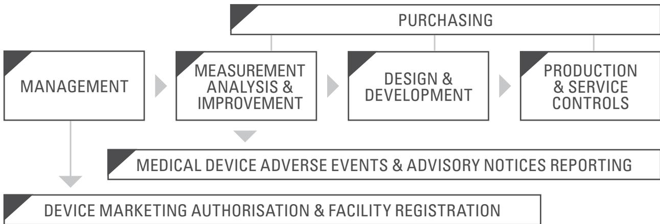
The flowchart shown in Figure 1, documents the MDSAP audit sequence and interrelationships. The MDSAP audit model was designed for the audit of the primary MDSAP processes in the following sequence: Management; Measurement, Analysis and Improvement; Design and Development; and Production and Service Controls.
