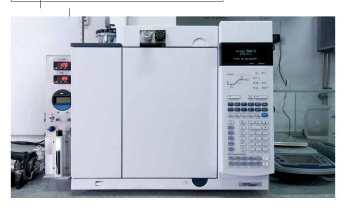
The SGS GC-GOR™ system is another example of innovation from ATIC. Every PVT laboratory uses a flash system of some sort and our laboratories are no different. However, we have designed a unique '0-flash system' that requires less sample volume, integrating the flash and compositional analyses into one unit. Unlike conventional systems where the flashed gas and oil are collected in separate vessels then
