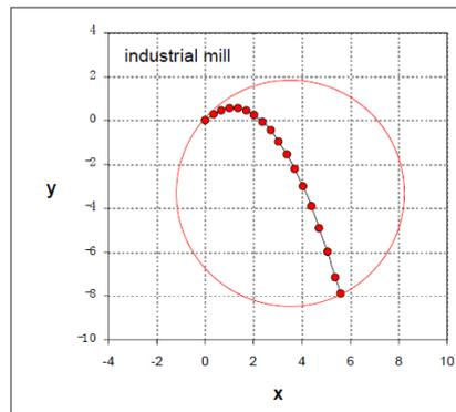
Figure 4 Ball trajectory (commercial mill)
