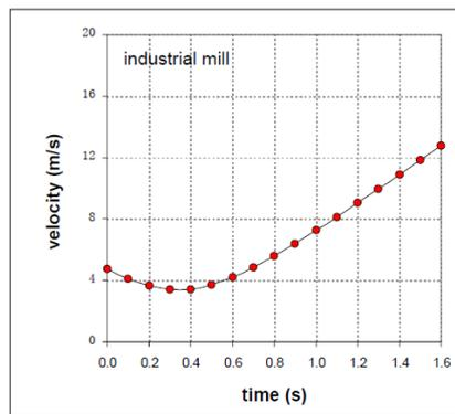
Figure 5 Impact velocity profile (commercial mill)
