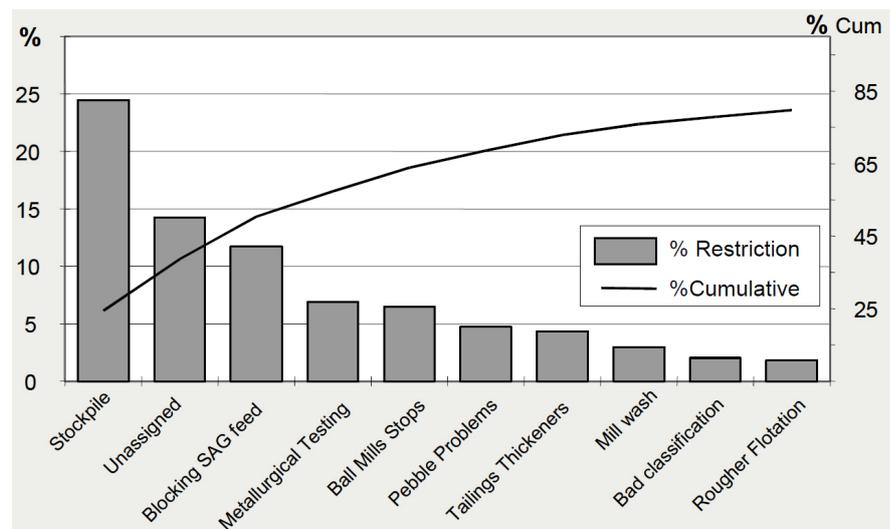
Figure 7: 80% of Los Colorados limitations not due to Ore hardness with impact Tph MEL Jul-Sep '03
