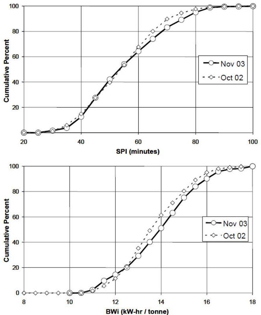
Figure 5: Distributions of SPI and BWi from 2002 and 2003 Hardness Models (after Preece, 2004<sup>B</sup>)
