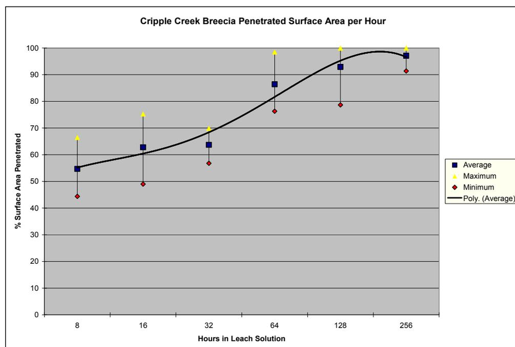
Figure 7: Penetration vs. Time for CCB
