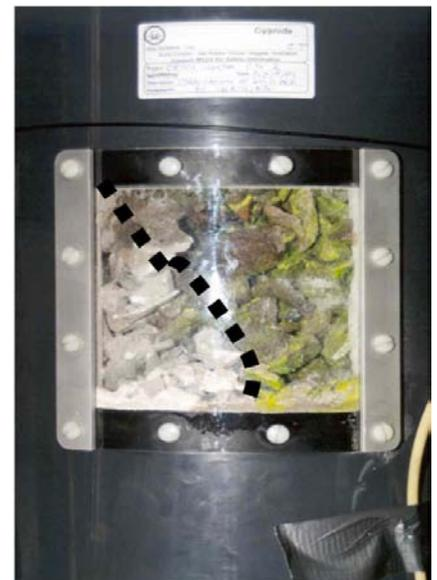
Figure 5: Photograph illustrating evidence of solution flow with dye added within hours of starting (Dashed line indicates solution horizon - solution on right / dry on left)
