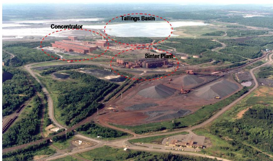
Figure 2 Overview of the "Cliff's Erie" Site Purchased by PolyMet Mining Corp. (This photograph was taken when the plant was producing taconite pellets seen in the foreground stockpiled ready for rail shipment.)
