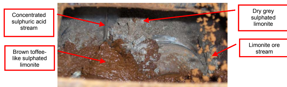
Figure 6 Photograph of Formation of Sulphated Limonite
