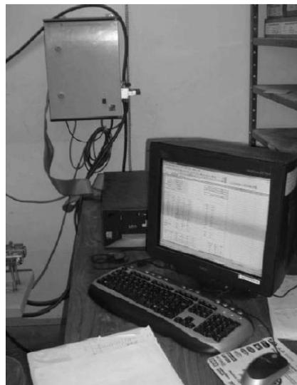
The computer data collection system allows accurate plots of distance vs. time, Figure 5 and force vs. time, Figure 6. The "knee" that occurs low down on the force vs. time plot appears to be the force needed to achieve full packing of the ore sample before any breakage begins, typically about 7.5 tons i.e. about 9 MPa in the 100mm diameter cylinder.
