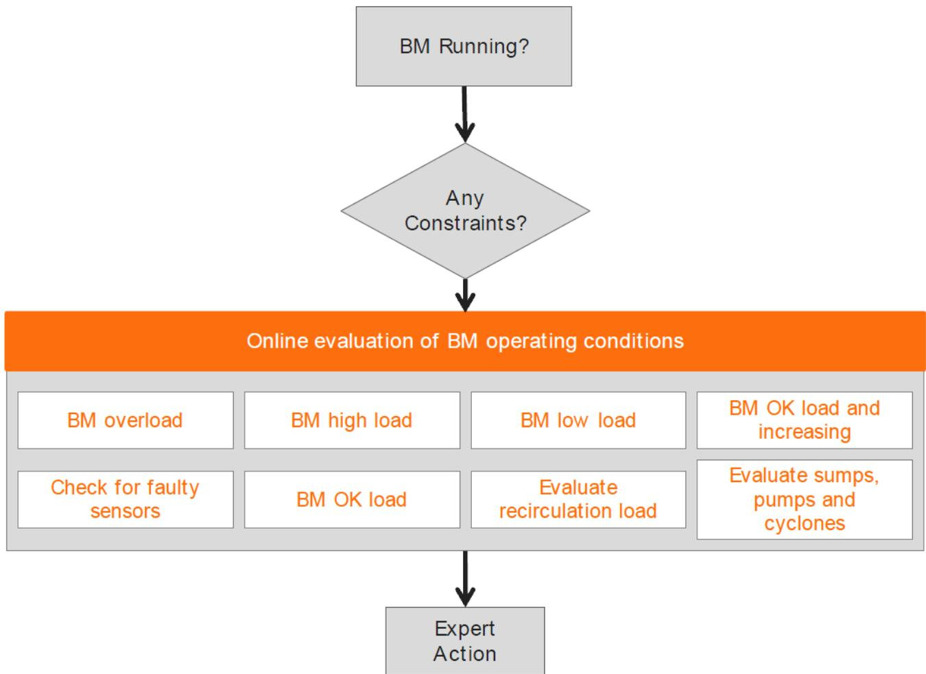
Figure 1. Primary Ball Mill Expert Logic Overview
