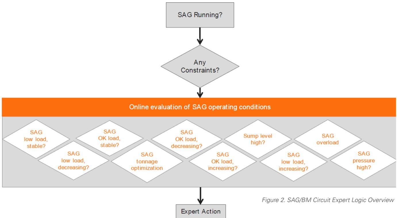
Figure 2. SAG/BM Circuit Expert Logic Overview
