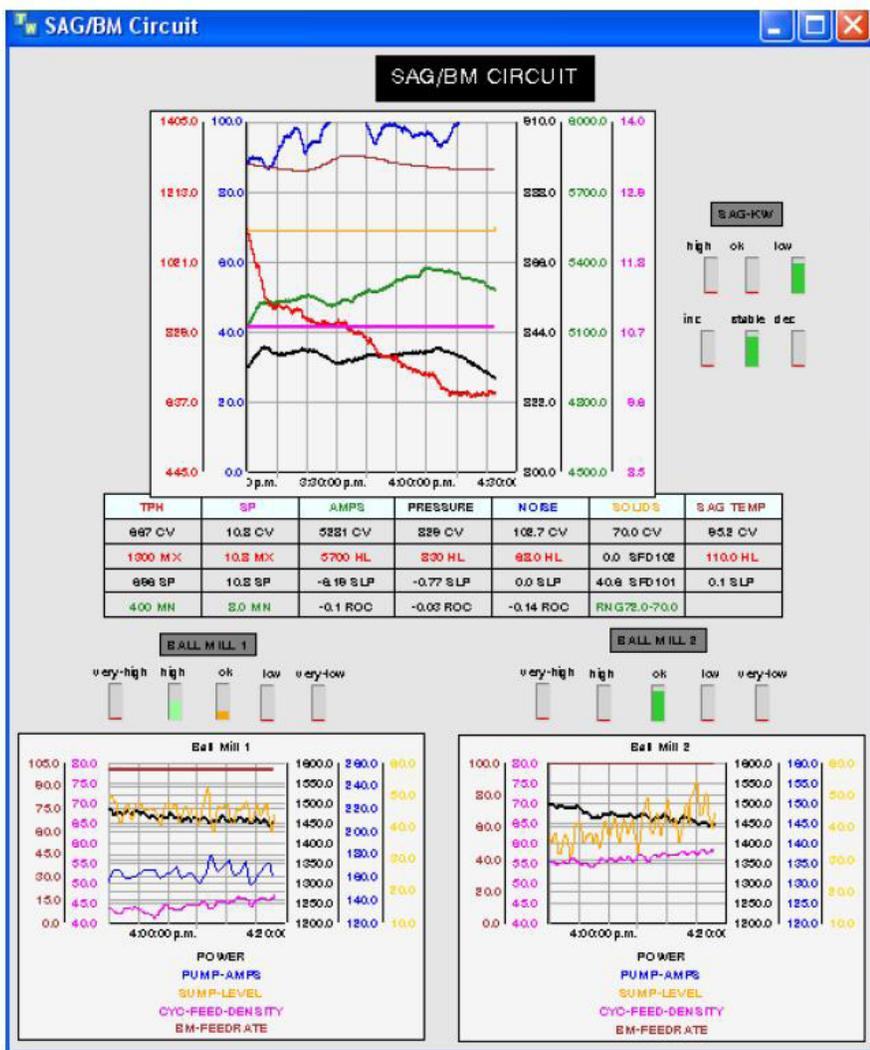
Figure 3. SAG/BM Circuit Expert Dashboard
