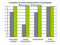
PEAR\* is a simplified life-cycle assessment for packaging that focuses on the most relevant stages of a packaging life cycle (manufacturing, transport, use, end of life) and draws conclusions on ten significant environmental impacts (climate, air, water, resources...).
